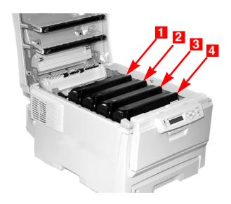
**3.** Lift the image drum, complete with its toner cartridge, out of the printer. Discard it in accordance with your local regulations.
